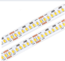
FITA DE LED | STRIP LED / 224 SMD 28*35 / PCB BRANCO | WHITE PCB / DIMERIZÁVEL | DIMMABLE / CRI>80
